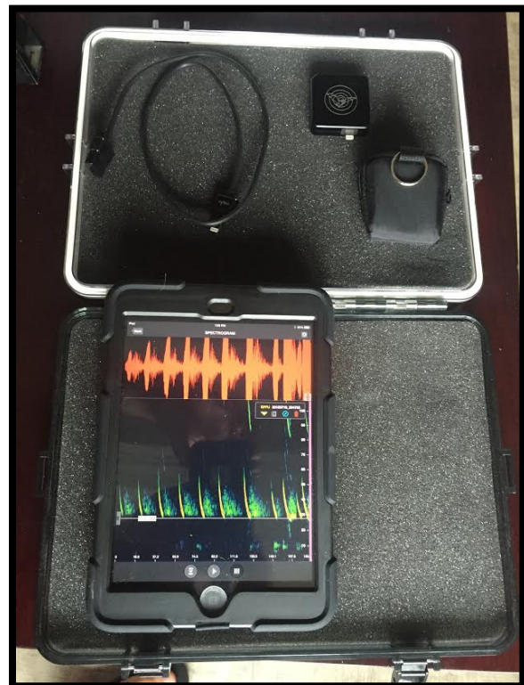
Figure 3. BatME detector kit. The iPad Mini is also depicting a representative screen shot from the EchoMeter App.
